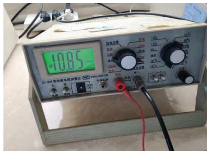
Gambar 2.7 Alat Mega ohmmeter tipe ZC-90E
