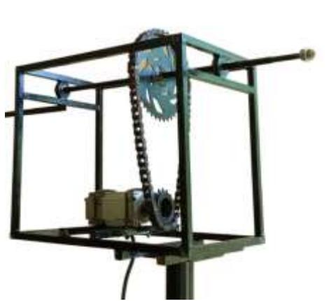
Gambar 4. 5 Rangka gearbox generator
