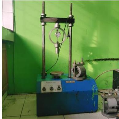
Gambar 3. 22 Alat uji Marshall
