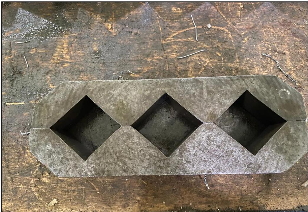
Gambar C.4 Persiapan Bekisting Kubus
