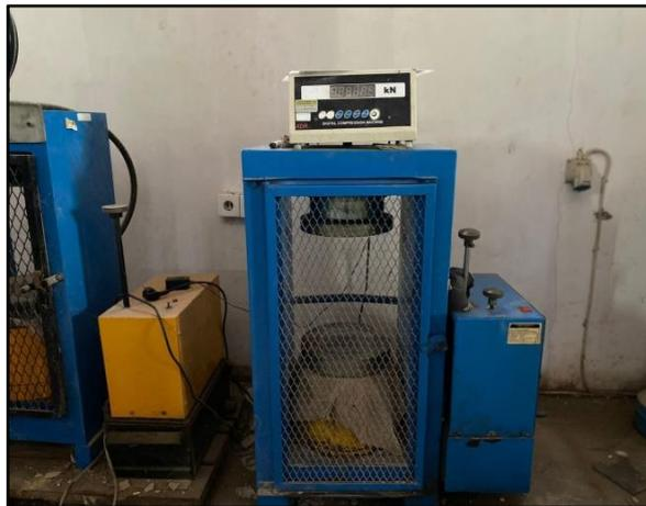
Gambar 3.14 *Compression testing machine*
