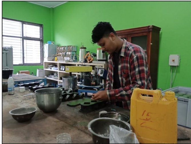
Gambar C.3 Persiapan Bekisting Kubus
