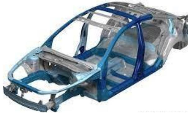
Gambar 2. 4 *Chassis Monocoque*
