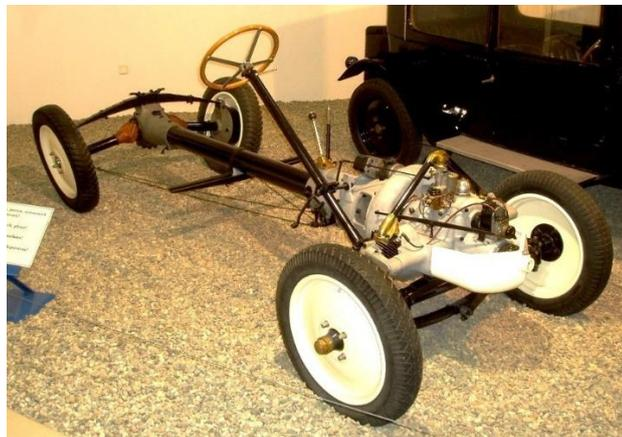
Gambar 2. 3 *Backbone chassis*
