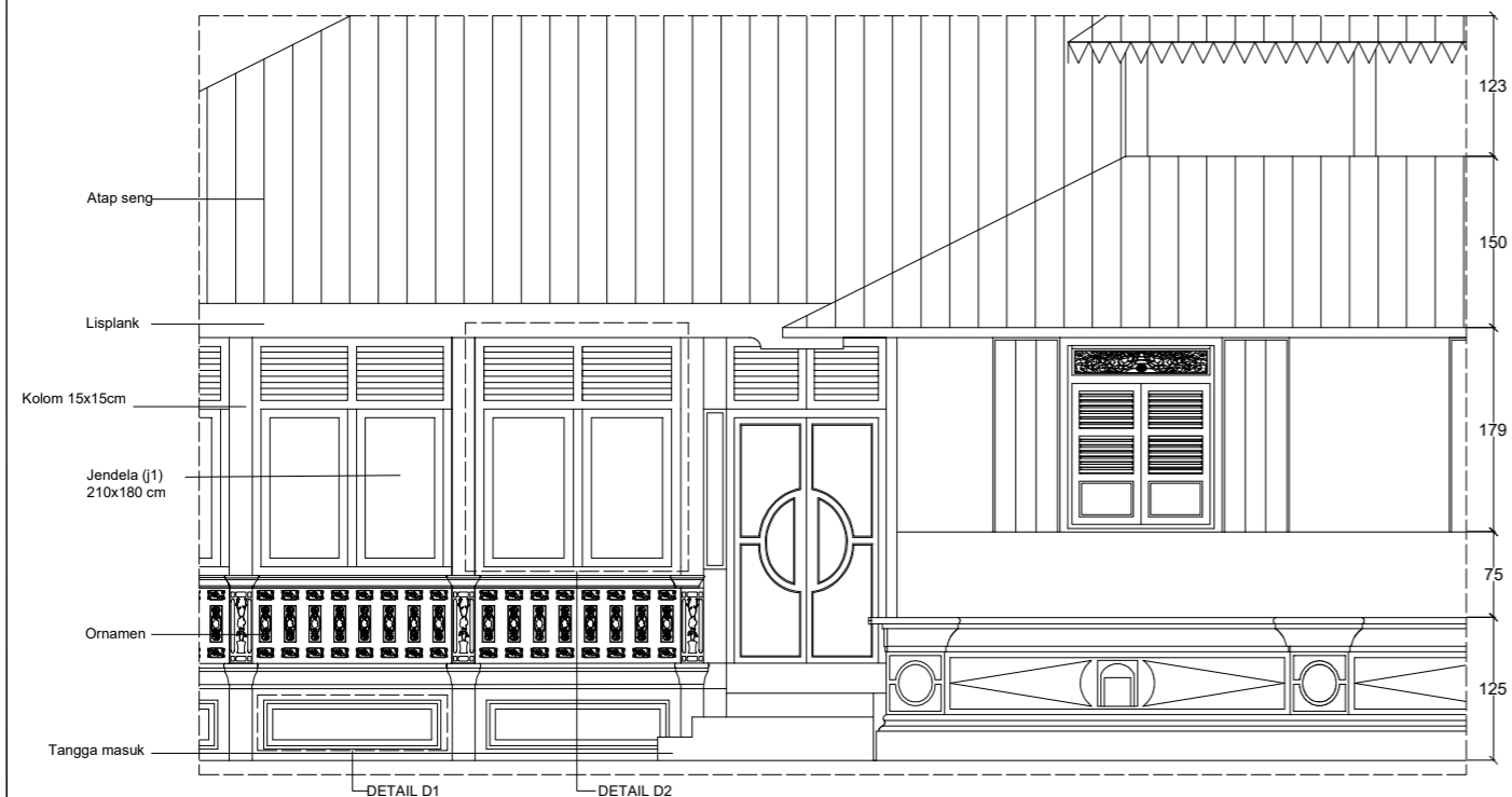
TAMPAK SAMPING KANAN (DETAIL D)
