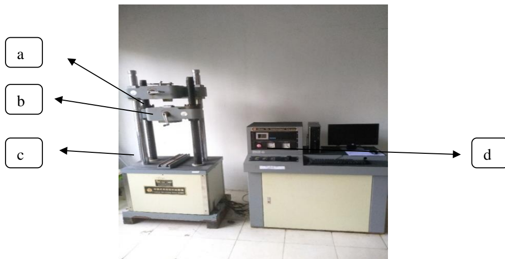
Gambar 3.5 Mesin uji tarik electro hydraulic servo type HT-9501. (Sumber : Laboratorium Teknik Mesin Unimal)
